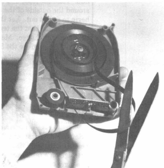
Tape is removed from its path and cut at splice.
