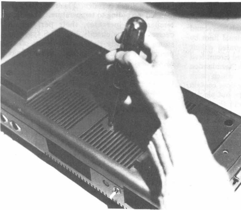
Photo 5-1. Photos on opening the expansion box. Screws are removed from bottom; note that like the CPU, a warranty-warning label may cover one screw.
