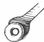
6. Bad solder connection - no contact with pin (SA sideview) (SB topview).
