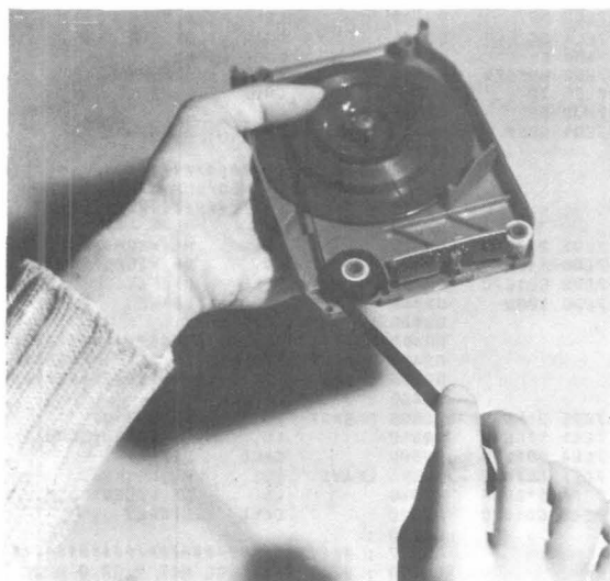
Excess tape is pulled gently from outside of the hub, letting hub and platter rotate freely. Note that end near center of hub has been cut fairly short to eliminate the possibility of tangling with the tape being removed.
