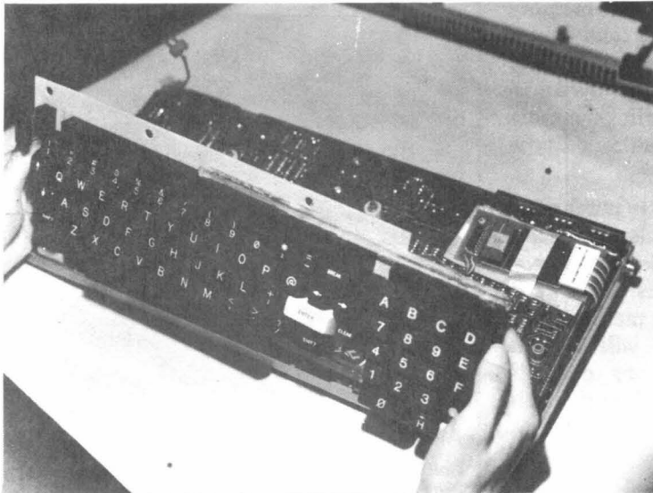
Keyboard is rocked gently forward to show white plastic spacers, which are then removed.
